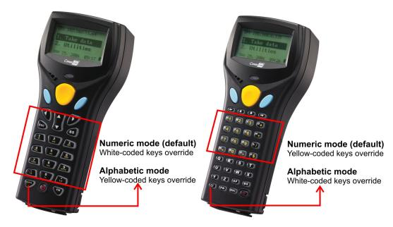
Figure 3: Keypad layout - 24-key (left), 39-key (right)
